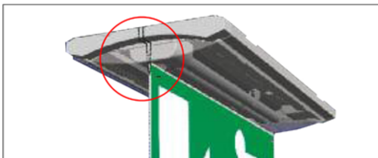
Quick lock in connection of the edgelit lens
